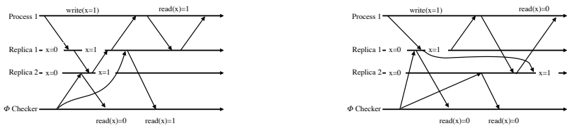
(a) Linearizable but not \phi -consistent execution. (b) \phi -consistent but not linearizable execution.
