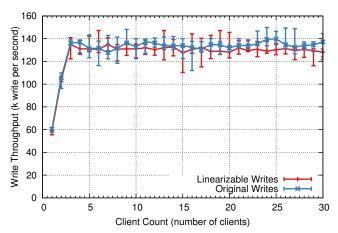
Figure 8: The aggregate throughput for one server serving 100B RAMCloud writes with and without RIFL, as a function of the number of clients. Each client repeatedly issued random writes back to back to a single server in a 4-server cluster. "Original Write" refers to the base RAMCloud system before adding RIFL. Each experiment was run 5 times. The data points show the median values; error bars show min and max.
