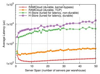
**Figure 13:** Average latency of TPC-C NewOrder transactions with a single warehouse, as a function of the degree of sharding for the warehouse. "Server Span" of 10 indicates that the data of a single warehouse is sharded across 10 servers. H-Store was tuned for low latency and measured with durability both enabled and disabled. RIFL-based transactions were measured on both RAMCloud's standard kernel-bypassing transport as well as over kernel TCP.
