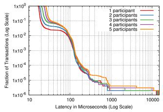
**Figure 10:** Reverse cumulative distribution of transaction commit latency measured from the beginning of the commit process to the completion of all prepare RPCs. Each transaction reads and writes one randomly chosen object per participant; the cluster contained 10 servers. A point (x, y) indicates that y of the 1M measured transaction commits took at least x µs to complete. The median latency for 1, 2, 3, 4, and 5 participants is 17.8 µs, 19.2 µs, 21.8 µs, 24.8 µs, and 27.3 µs respectively.
