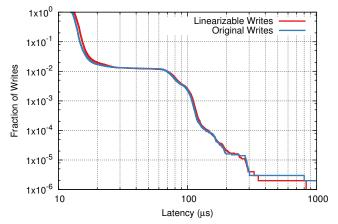
**Figure 7:** Reverse cumulative distribution of latency for 100B random RAMCloud write operations with and without RIFL. Writes were issued sequentially by a single client to a single server in a 4-server cluster. A point (x, y) indicates that y of the 1M measured writes took at least x µs to complete. "Original Write" refers to the base RAMCloud system before adding RIFL. The median latency for linearizable writes was 14.0 µs vs. 13.5 µs for the original system.
