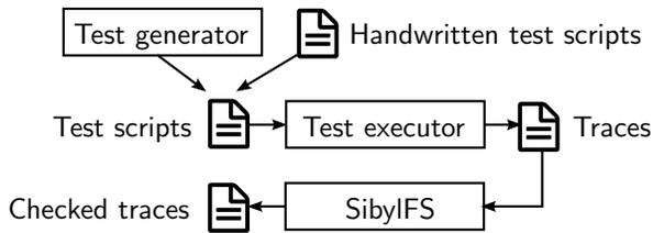
**Figure 1.** File system testing and trace checking
