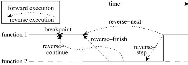
**Figure 2: The reverse analogs of standard debugging commands.**
